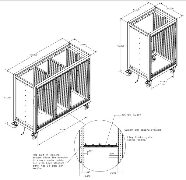
Available in 30" and 60" widths, Solder Pallet Carts come standard with two fully adjustable end panels with a built-in indexing system that makes finding the right slot easy. Optional double-sided panels may be added to increase solder pallet capacity. Custom slot spacing available.
